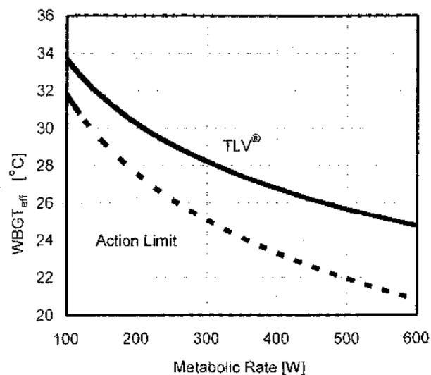
**FIGURE 2.** TLV<sup>®</sup> (solid line) and Action Limit (broken line) for heat stress. WBGT<sub>eff</sub> is the measured WBGT plus the Clothing-Adjustment Factor.
